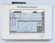
The Pile Dynamics Analyzer - Dynamic Load Tester was designed specifically for quality assurance testing of drilled shafts, bored piles, ACIP/CFA piles, as well as other applications. This system acquires data from accelerometers and strain transducers attached to a pile or shaft so High Strain Dynamic Testing may be performed. Customize the system to best suit your project, with cabeled and wireless options.
